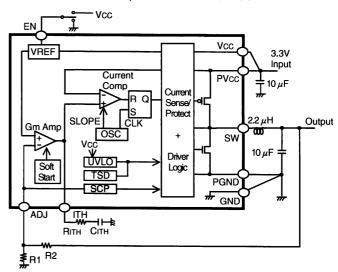
The Output Voltage is set by the external resistor divider and is calculated as:  $Vout=(R2/R1+1)\times VADJ \quad \bullet \quad \textcircled{1} \quad VADJ : ADJ \text{ pin reference Voltage } (0.8V \text{ typ})$  It's possible to adjust the output voltage by R1 and R2. (The Vout must be set from 1.0V to 2.0V.) Resistance R1  $\stackrel{\leftarrow}{=}$  10k  $\Omega$  is recommended. Please confirm the ripple voltage, if you can use the resistance more than  $100\text{k}\,\Omega$ .
