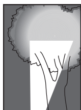
Uplighting from below makes details stand out
