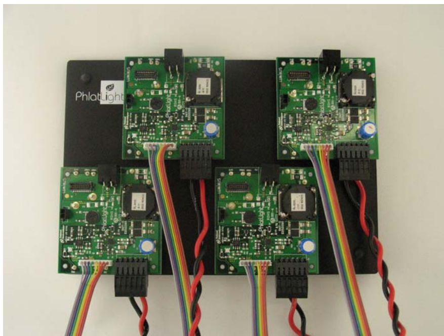
Figure 5: Completed electrical connections on DK-414N-4
