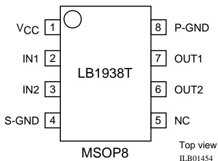
S-GND: GND for the control system
