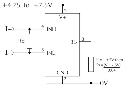
Measuring a current from a circuit which is floating with respect to the DPM's supply, i.e. the current and the meter's power supply are isolated from each other.
