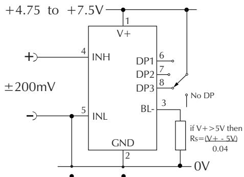
Measuring a single ended input voltage referenced to supply, i.e. the input voltage and the meter's power supply share the same 0V rail.
