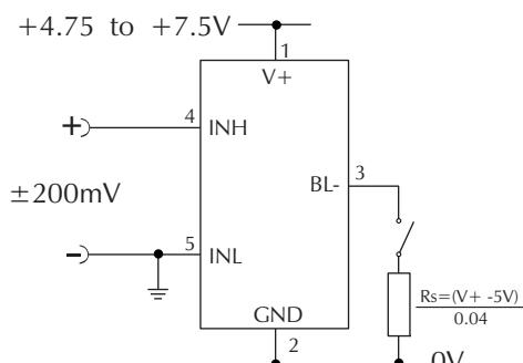
Measuring a single ended input voltage referenced to supply, i.e. the input voltage and the meter's power supply share the same 0V rail.
