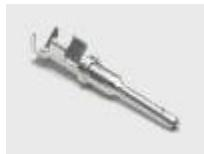
1060-16-0122-PS Pin, Stamped and Formed, Nickel, 14-18 AWG, .075-.140 Insulation
