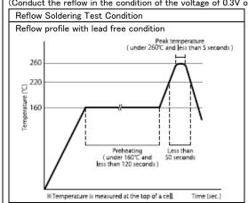
Cautions: Do not charge prior to reflow, Set reflow condition within the range provided in "Specifications", which will be published separately
