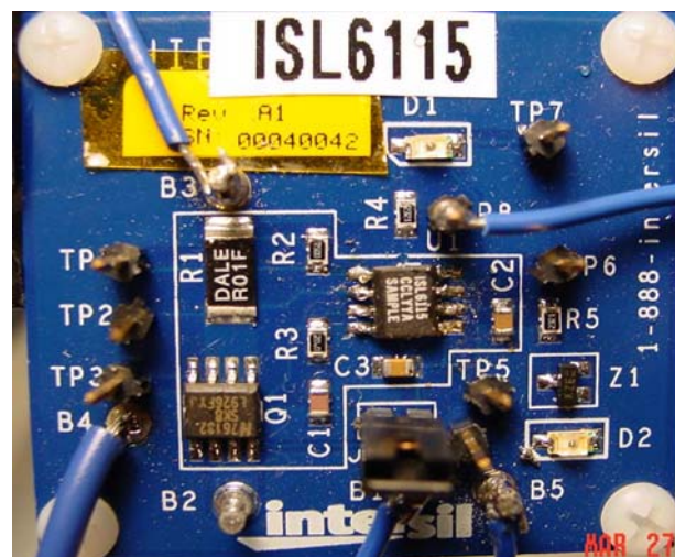
FIGURE 18. ISL6115 EVAL BOARD PICTURE
