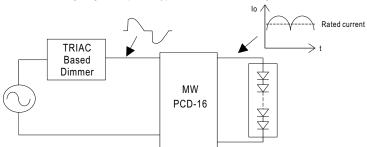
Under direct driving, the power supply will work in "constant current mode (CC)" and output voltage of the power supply will be clamped by sum of forward voltage (VF) of the LED strip.
