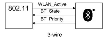
In order for any of these schemes to operate, it requires the appropriate, complementary algorithms to be implemented and activated in both devices. Simply connecting up signal lines will not result in any co-location strategies being used.
