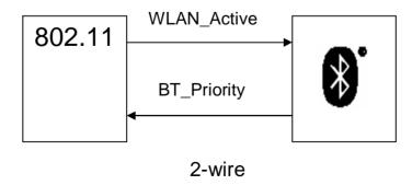
In 2-wire schemes, only two signals are used to connect the Bluetooth and 802.11 sections. These typically convey the status of the wireless LAN
