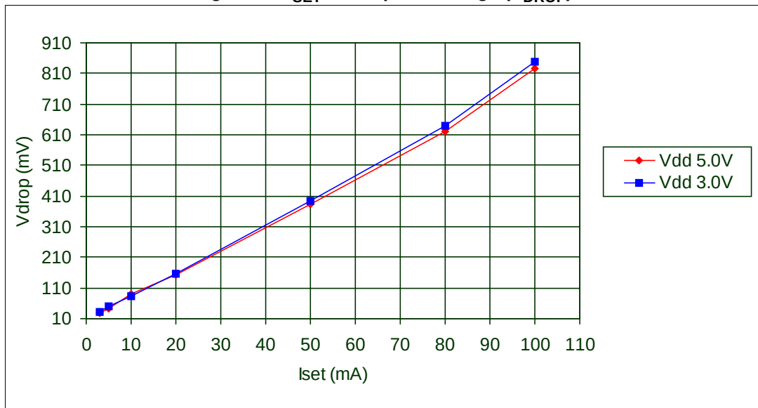
Figure 12. I_{SET} vs drop out voltage ( V_{DROP} )
