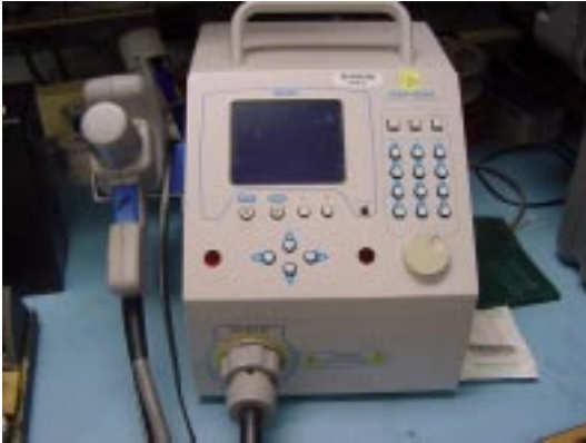
Figure 9. ESD Generator, NoiseKen ESS-2000
