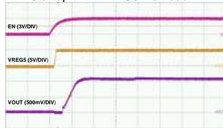
Startup with VREG5 No Load
