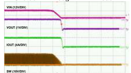
Shutdown Through VIN 4A Load
