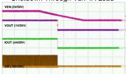
Shutdown Through VEN 4A Load
