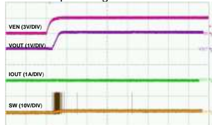
Startup Through VEN No Load
