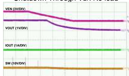
Shutdown Through VEN No load
