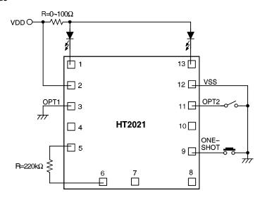
\* The IC substrate should be connected to VDD in the PCB layout artwork.
