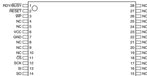
TSOP Top View Type 1
