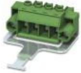
PCB connector, nominal current: 41 A, rated voltage (III/2): 1000 V, nominal cross section: 6 mm<sup>2</sup>, number of positions: 2, pitch: 7.62 mm, connection method: Screw connection with tension sleeve, color: green, contact surface: Tin
