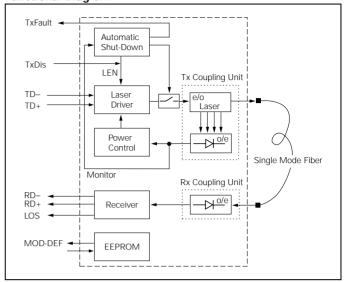
The receiver component converts the optical serial data into PECL compatible electrical data (RD+ and RD-). The LOS of Signal (LOS, active low) shows whether an optical signal is present.
