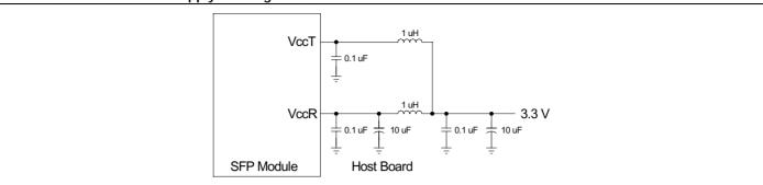
**Example SFP Host Board Schematic**
