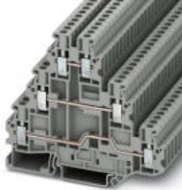
Multi-level terminal block, Cross section: 0.14 mm<sup>2</sup> - 4 mm<sup>2</sup>, AWG: 26 - 12, Connection type: Screw connection, Width: 5.2 mm, Color: gray, Mounting type: NS 35/7.5, NS 35/15
