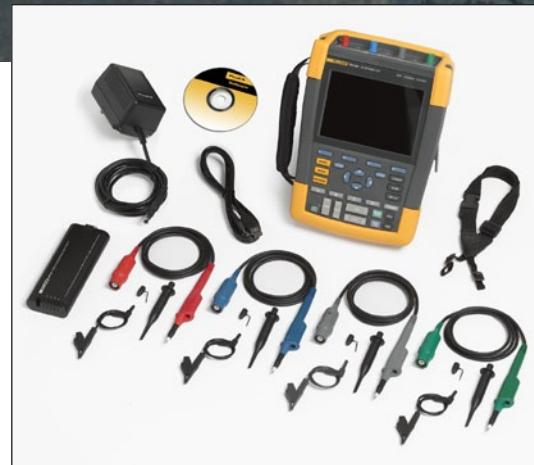
Fluke 190 Series II instruments include a set of voltage probes (2 or 4 dependant on model), hanging strap, USB cable with mini-B connector, double capacity Li-Ion battery BP291, battery charger/power adapter BC190, a FlukeView demo package and user manuals on CD.
