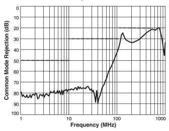
802.3af specification: 50 dB min from 1 MHz to 10 MHz 30 dB min from 10 MHz to 125 MHz
