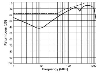
802.3af specification: 18 dB min from 1 MHz to 40 MHz 16 dB min at 50 MHz 12 dB min at 80 MHz 10 dB min at 100 MHz
