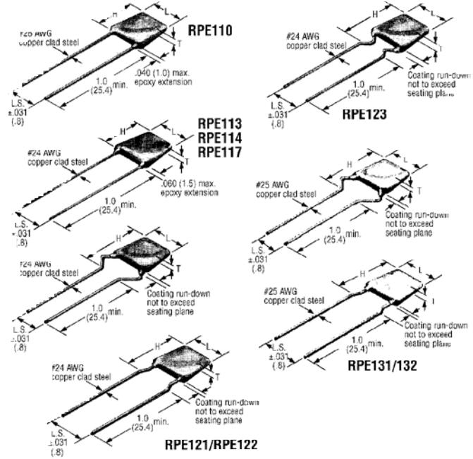
These monolithic ceramic capacitors have industry standard sizes and an epoxy coating meeting UL94V-0. Leads are tinned copper clad steel wire. Additional values, voltages, temperature coefficients, tolerances and markings available, as well as additional lead spacing and tape and reel option available as custom order. Call for price and delivery.
