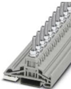
High Current Connectors, nom. voltage: 1000 V, nominal current: 76 A, connection method: Bolt connection, number of connections: 1, width: 13 mm, height: 56.1 mm, color: gray, mounting type: NS 35/7,5, NS 35/15
