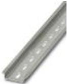
DIN rail perforated, Standard profile, width: 35 mm, height: 7.5 mm, acc. to EN 60715, material: Steel, galvanized, passivated with a thick layer, length: 2000 mm, color: silver
