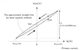
• When  $Ip_{(RMS)}$ max is bigger than the value of If,  $Ip_{(RMS)}$ max restricts it to the value of If.
