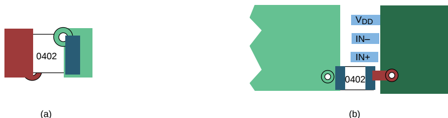
Figure 48. Typical Decoupling Capacitor Layouts
