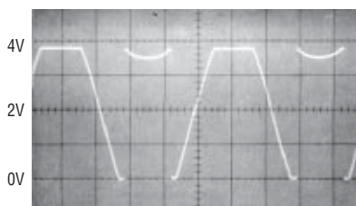
LM324, LM358, OP-20 EXHIBIT OUTPUT PHASE REVERSAL
