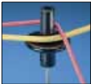
In the "up" position to form harness.
