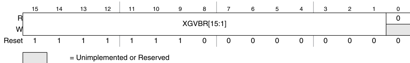
Figure 10-9. XGATE Vector Base Address Register (XGVBR)
