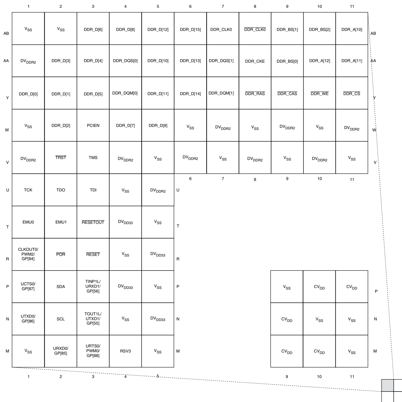
Figure 2-10. ZDU Pin Map [Quadrant A]
