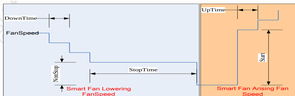
Figure 6-1 SMART FAN™ IV Control Parameters
