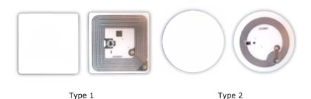
Type 1 tag is based on ISO/IEC 14443A standard and has 512 bytes of memory. Type 2 tag is based on ISO/IEC 14443A standard and has 192 bytes of memory.
