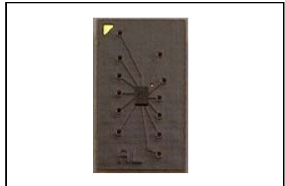
FIGURE 1. CSP TO DIP CONVERTER BOARD
