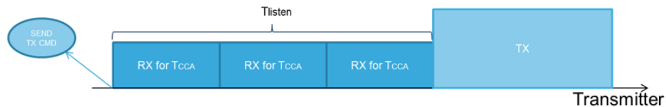
Figure 23. CSMA if channel is free (timeline)
