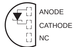
LP (TO-92/TO-226) PACKAGE (TOP VIEW)
