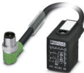
Sensor/Actuator cable, 3-position, PUR halogen-free, Black-gray RAL 7021, Plug angled M12 SPEEDCON, A-coded, on Valve connector BI (11 mm), with 1 LED, connected with Z diode, Cable length: 7.5 m
