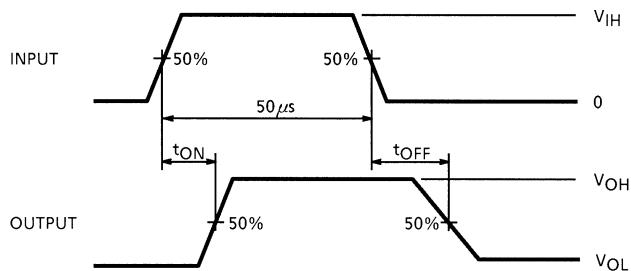
Note 1: Pulse width 50  $\mu$ s, duty cycle 10%
