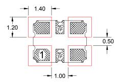
Note: XpressO HCMOS XO's are designed to fit on industry standard, 4 pad layouts.
