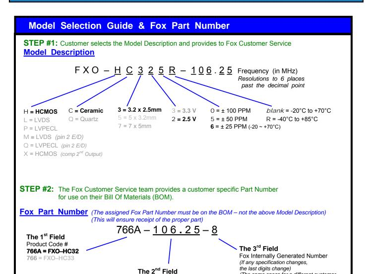
This example, FXO-HC325R-106.25 = HCMOS Output, Ceramic 3.2 x 2.5mm Package, 2.5V, ±50 PPM Stability, -40 to +85°C Temperature Range, at 106.25 MHz
