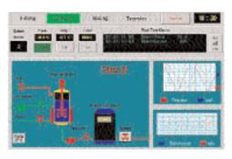
The LNS DDE Server is an I/O driver for human-machine interface (HMI), supervisory control and data acquisition (SCADA), operator interface, and visualization applications. The LNS DDE Server is not required by the NodeBuilder software, but it provides an easy and high-performance way to access your LonWorks networks and devices from applications that support a DDE, Fast DDE, or SuiteLink interface such as Wonderware® InTouch®, Intellution Fix, or National Instrument BridgeView and LabView.
