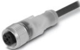
Sensor/Actuator cable, 3-position, PUR halogen-free, Black-gray RAL 7021, Free cable end, on Socket straight M12, A-coded, Cable length: 5 m
