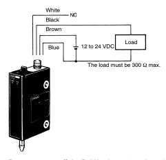
Be sure to turn off the D5VA when wiring the cable connected to the D5VA or connecting or disconnecting the connector to or from the D5VA, otherwise the D5VA or load may malfunction or be damaged.
