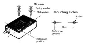
Mount the D5V with M4 screws, flat washers, and spring washers securely. Tighten each M4 screw to a torque of 1.18 to 1.47 N  $\bullet$  m (12 to 15 kgf  $\bullet$  cm).
