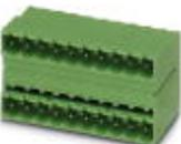
Header, Nominal current: 10 A, Rated voltage (III/2): 320 V, Number of positions: 16, Pitch: 5 mm, Color: green, Contact surface: Tin, Assembly: Soldering, In combination with MVSTB or FKCV plug components, both an MVSTBW (or FKCVW) and an MVSTBR plug (or FKCVR) must be used. Combination with TMSTBP plug components is not possible!
