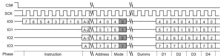
Figure 77. Quad I/O Read Command Sequence (EBh or ECh)
