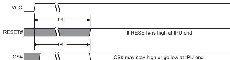
Figure 24. Reset High at the end of POR
