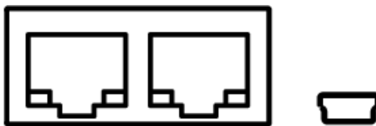
Figure 20: Network and USB Connectors
