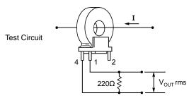
The CS60 Series measures current from 5 to 100 amps rms. Applications include sensing branch circuit overload and detecting load drop or shutdown. The sensor functions as the encapsulated secondary of a current transformer, while the conductor carrying the current to be measured serves as the "one turn primary." Sensitivity may be enhanced by increasing primary turns.
