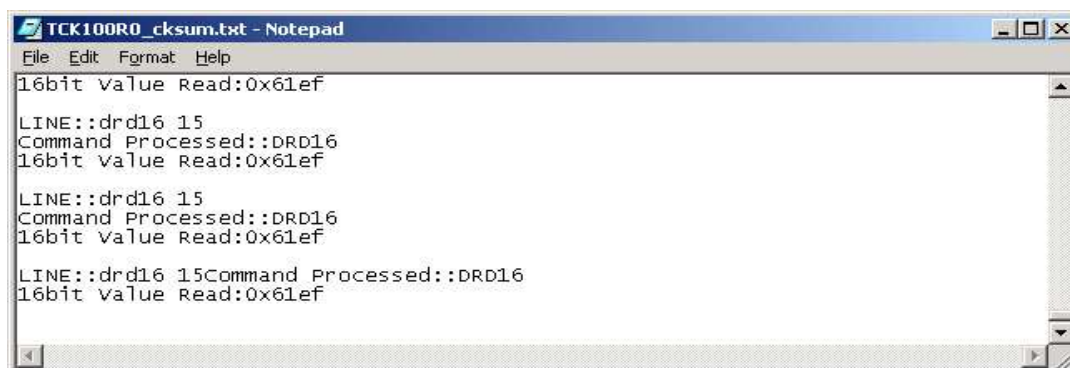
Figure 2-19. Checksum File Showing the Generated Checksum Result (0x61ef) from Configuration File gc5016_diagtest2.dat
