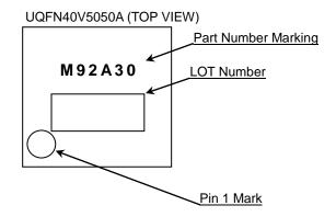
**Physical Dimension and Packing Information** Package Name UQFN40V5050A 5.0±0.1 0±0 1PIN MARK 0.035 -0:018 (0.203) 0.08S CO.2 3.6±0.1 40 Detail A 4±0. 0.282 Ö 0.082 31 30 0.2±0.05 0.4 (U I NT : mm) PKG: UQFN40V5050A Drawing No. EX001-0014 <Tape and Reel information> Tape Embossed carrier tape 2500pcs Quantity Direction The direction is the 1pin of product is at the upper left when you hold reel on the left hand and you pull out the tape on the right hand of feed
