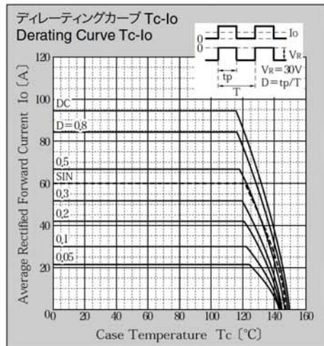
\* Sine wave is 50Hz used for measurements.
