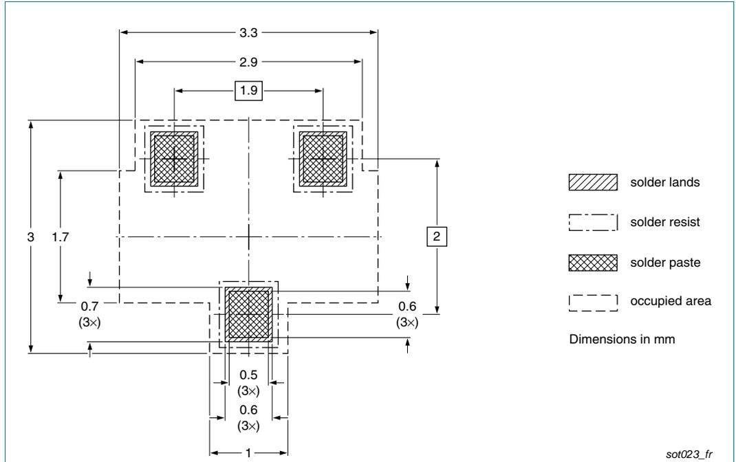
**Fig 9. Reflow soldering footprint PMBD7000 (SOT23/TO-236AB)**
