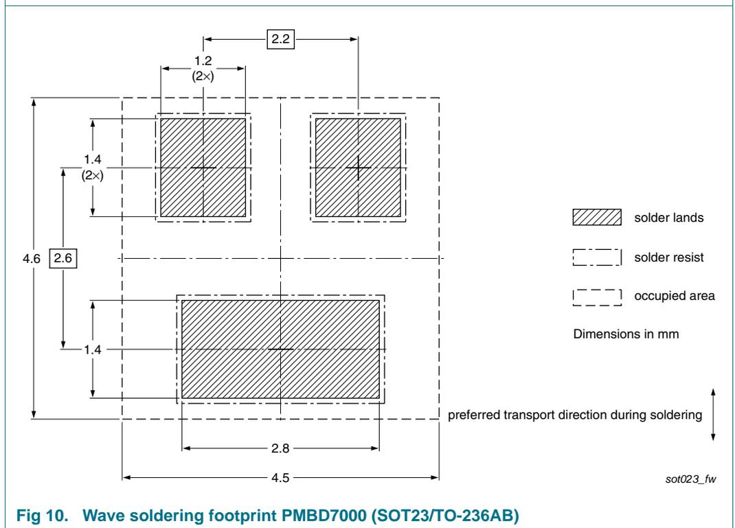
**Fig 10. Wave soldering footprint PMBD7000 (SOT23/TO-236AB)**
