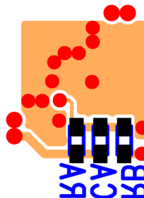
Figure 5: Bottom PCB Layer Critical Components (RA, RB, CA) & Copper for Minimum Footprint
