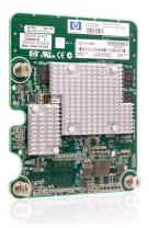
NC522m Intelligent Ethernet Adapter. The NC522m is a dual port, IEEE 10GBase-KR 10-Gigabit Ethernet network adapter for the HP ProLiant c-Class BladeSystem. This adapter is based on the QLogic NX3031 controller.
