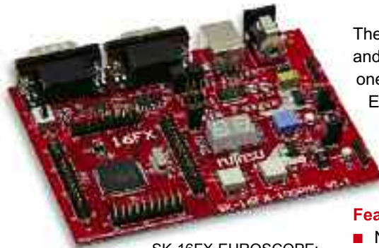
SK-16FX-EUROSCOPE: On-chip debugger with target board.
