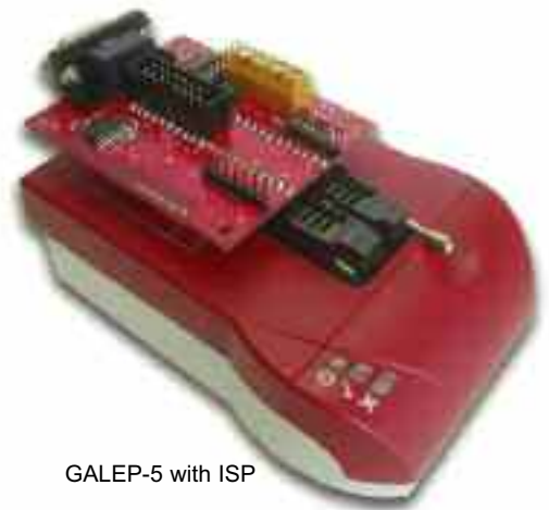
GALEP-5 is a professional palm-sized field programmer with universal I/O capability
